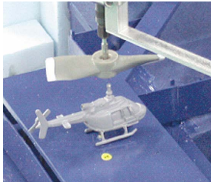
Figure 2: Wind tunnel testing of helicopter model
