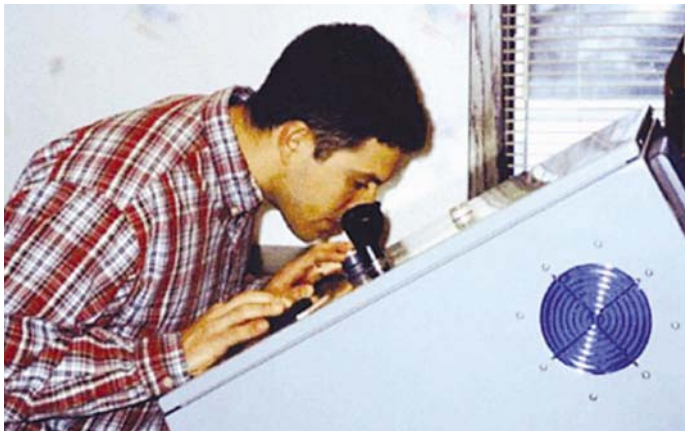
Odor panel testing used to establish design criterion
