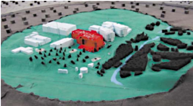
Scale model of a site with complex topography simulated in a boundary layer wind tunnel.
