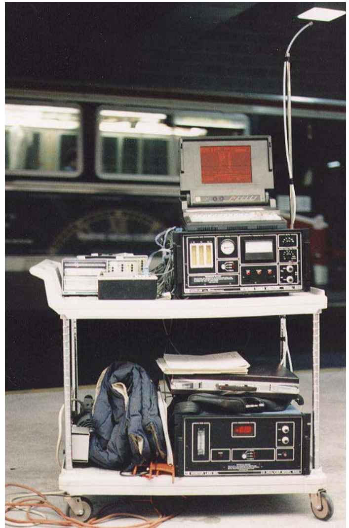
Continuous indoor air quality monitoring system in a bus terminal
