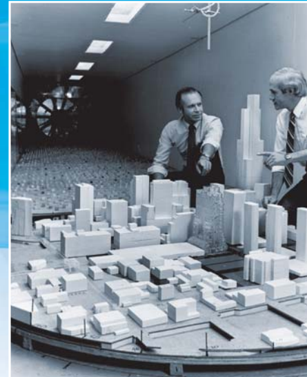
Bill Rowan (left) and Peter Irwin review model in second boundary layer wind tunnel
