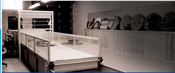
The open channel water flume – the “wind and snow simulator”
